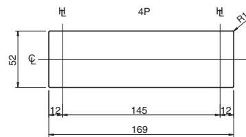
The cutout dimensions allow for a side clearance of 1.0 mm from the bank of the breaker.
