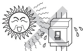
Install the breakers in an area that is not exposed to direct sunlight.
